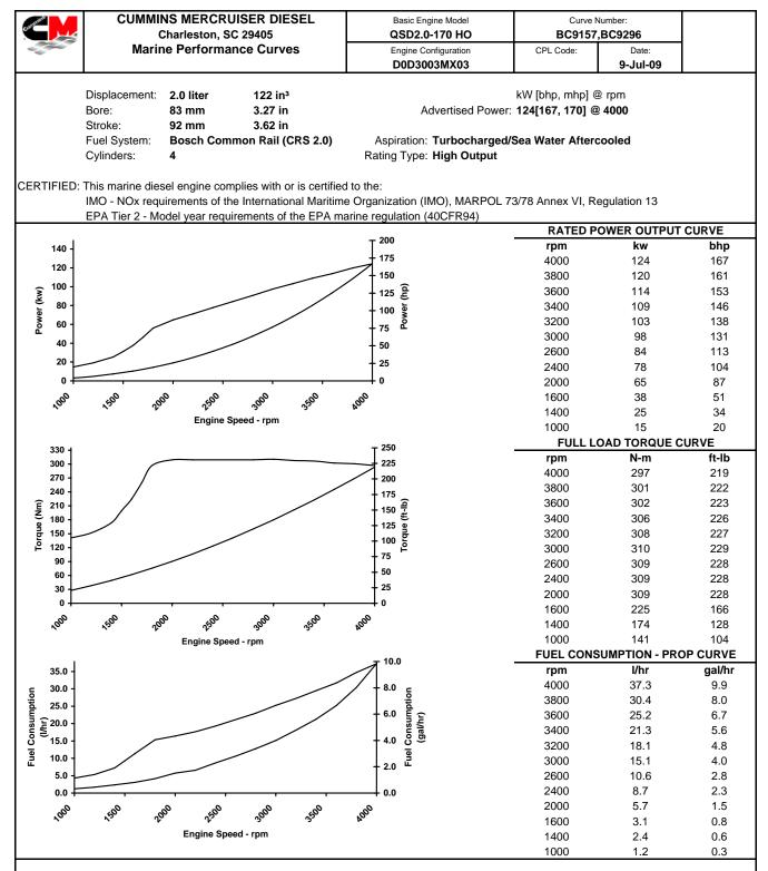
Rated Conditions: Ratings are based upon ISO 15550 reference conditions; air pressure of 100 kPa [29.612 in Hg], air temperature 25deg. C [77 deg. F] and 30% relative humidy. Power is in accordance with IMCI procedure. Member NMMA.
